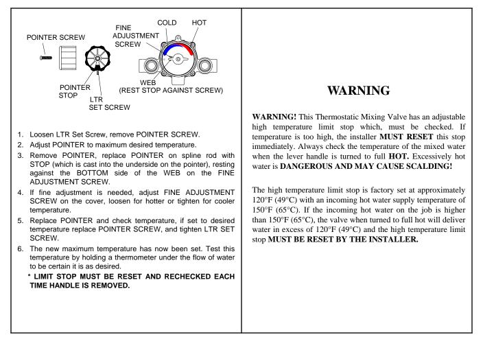
Check for significant variations in outlet flow. Thermostatic valves will NOT provide the desired accuracy outside of their flow capacity range. Minimum flows must be no less than shown (see Flow Capacities, page 6).
